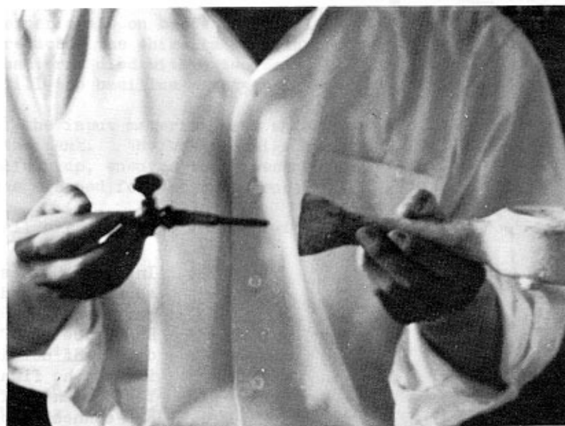
Plate 31. Showing the nozzle which fits into the clay biogas burner of Plate 30.
